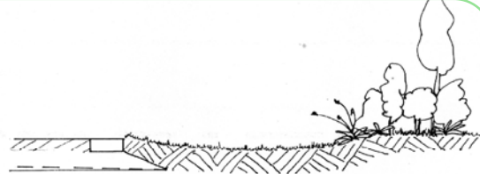
Section through grassed 2500 swale
